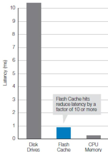
**Figure 2) NetApp Flash Cache intelligent caching optimizes performance for business analytics.** By using controller-attached PCIe intelligent caching instead of more hard disk drives, Flash Cache improves storage I/O for random read-intensive workloads, reducing latency by a factor of 10 or more.
