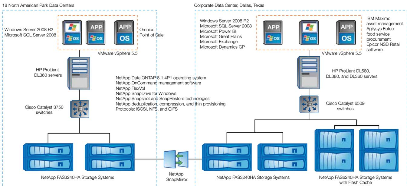
**Figure 1) Six Flags Entertainment's NetApp storage infrastructure.** Identical mini data centers at 18 theme parks replicate data back to the primary data center in Dallas by using NetApp SnapMirror® technology.
