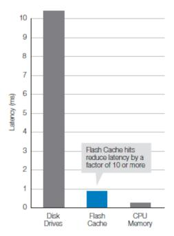
Figure 2) NetApp Flash Cache intelligent caching optimizes performance for business analytics. By using controller-attached PCle intelligent caching instead of more hard disk drives, Flash Cache improves storage I/O for random read-intensive workloads, reducing latency by a factor of 10 or more.
