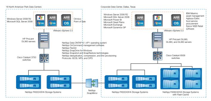
Figure 1) Six Flags Entertainment's NetApp storage infrastructure. Identical mini data centers at 18 theme parks replicate data back to the primary data center in Dallas by using NetApp SnapMirror® technology.
